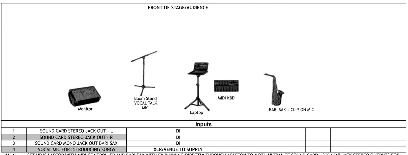
Notes: SET UP IS LAPTOP WITH MIDI CONTROLLER AND BARI SAX WITH FX RUNNING DIRECTLY THROUGH ABLETON TO MOTU ULTRALITE SOUND CARD - 2 X 1/4" JACK STEREO OUTPUTS FOR LAPTOP AND 1 X 1/4" JACK OUTPUT FOR BARI SAX FX CHANNEL
